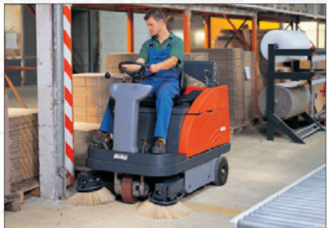
Hako-Jonas 980 E: For exhaust-free indoor applications with electric drive and different types of battery system. Running time up to 4,5 hours.
